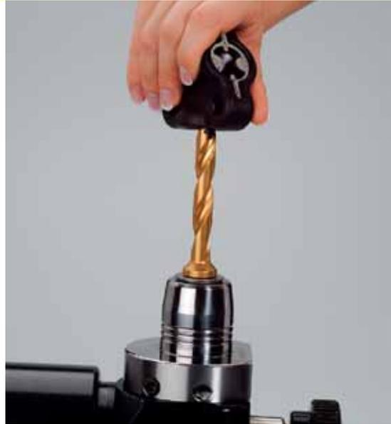
Simple and high-precision head replacement due to centre bore in the main body and stud in the carbide head: Insert head, turn slightly (picture left) and fix with key (picture right).
