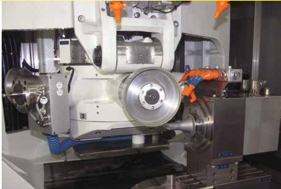
**Working area of the 6-Axis grinding machine.**
