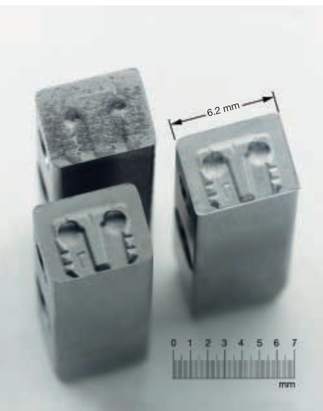
Geometry male dies machined with micro milling process for inserts type S224 and S229
